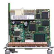
Rear Accessible M100 Shelf Management Module
